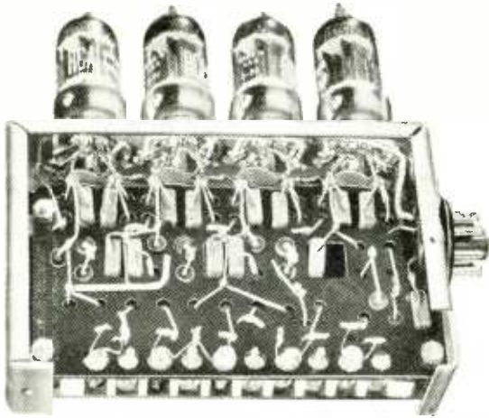
Fig. 3. Decade counter of the type described, built as a plug-in unit for use in a commercial instrument.
