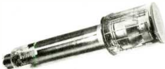
English Electric 4½ in image orthicon camera tube.
