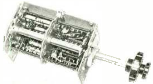
Turret of Ediswan-Clix television tuner with some coil units removed to show interior.
